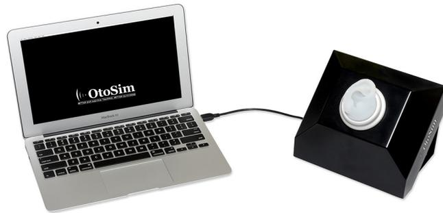
The OtoSim™ Base Unit can be connected to a desktop computer or a laptop by inserting the Type A (larger) end of the USB cable into the port on the computer.
