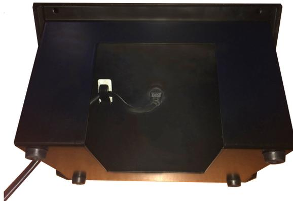
The USB port is located on the backside of the Base Unit. Insert the Type Mini B (smaller) end of the USB cable into the port on the Base Unit.
