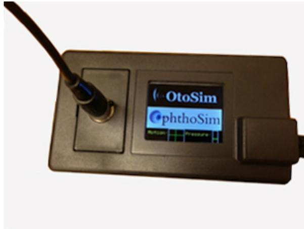
**Note:** The two graphs at the bottom of the screen are intended solely as a diagnostic to verify that all the tracking circuitry is functioning correctly. If you do not see any motion when you move the otoscope, the Sensor Box may be malfunctioning. If the Base Unit displays “Not connected”, then you should ensure the cable between the Sensor Box and the Instrumented Otoscope is snugly connected and undamaged.
