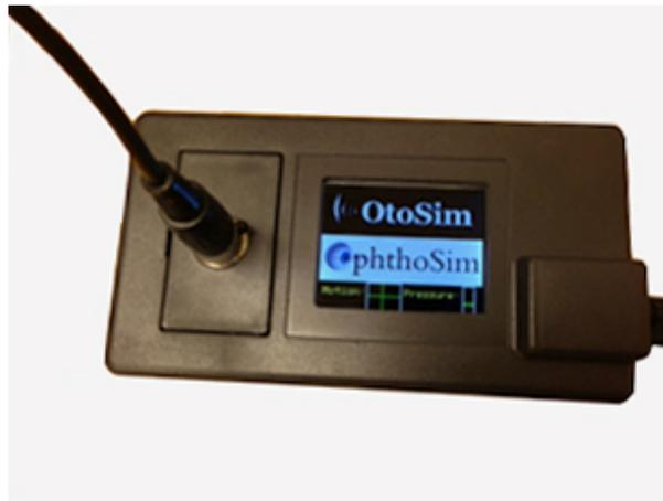
**Note:** The two graphs at the bottom of the screen are intended solely as a diagnostic to verify that all the tracking circuitry is functioning correctly. If you do not see any motion when you move the ophthalmoscope, your unit may be malfunctioning. If your unit displays “Not connected”, then you should ensure the cable between the Sensor Box and Ophthalmoscope is snugly connected and undamaged.
