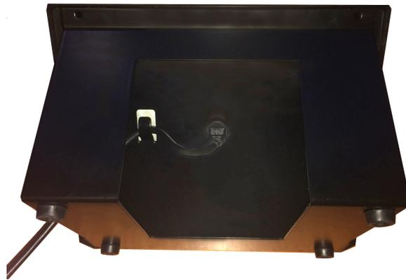
The USB port is located on the backside of the Base Unit. Insert the Type Mini B (smaller) end of the USB cable into the port on the Base Unit.
