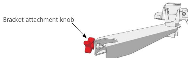
3. On the cart mount or the IV pole mount, ensure that the locking pin and quick-release lever are in the unlocked (horizontal) position.
