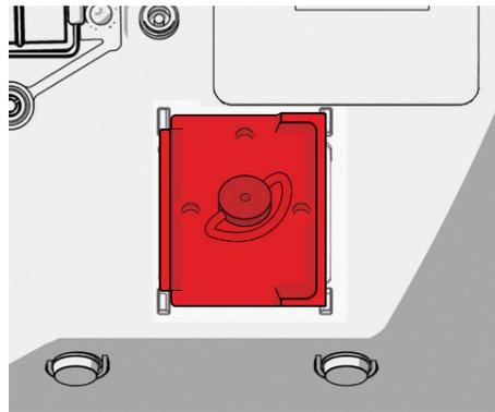
5. Seat the locking plate of the monitor on the quick-release mount. When properly situated, the monitor sits securely on the mount, and the quick-release lever automatically snaps into the locked (down) position.
