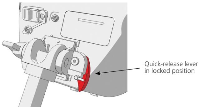
7. Adjust the locking pin to the locked (down) position. This secures the quick-release lever in the locked position.
