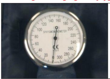
Make sure gauge is set at zero. If the gauge is not at zero, a needle-nose pliers can be used to calibrate it. Locate the two flat spots on the end of the gauge; slowly turn clockwise or counterclockwise until the needle is set at zero.
